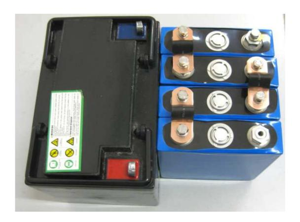
The 4 pieces WN-36AH cells can also simply replace the 12V starting battery in a conventional car.
