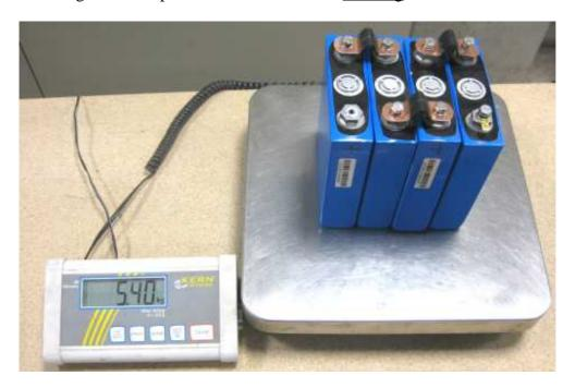
The weight of the 12V battery made of WN-36AH is 46% of the SLA battery.
